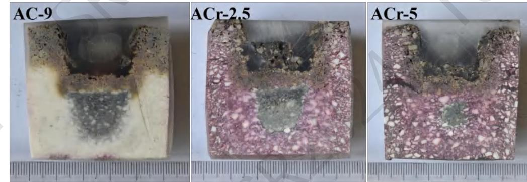
Cross-section of the samples with different  $\text{Cr}_2\text{AlC}$  contents after the corrosion test at  $1600^\circ\text{C}$
